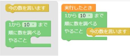
A Scratch script for Stage 4. It consists of a yellow 'say' block with the text '今の数を言います', a green 'loop' block with '1から 10 まで' and '順に数を調べる やること', and an orange 'when green flag clicked' block with the text '今の数を言います'.
